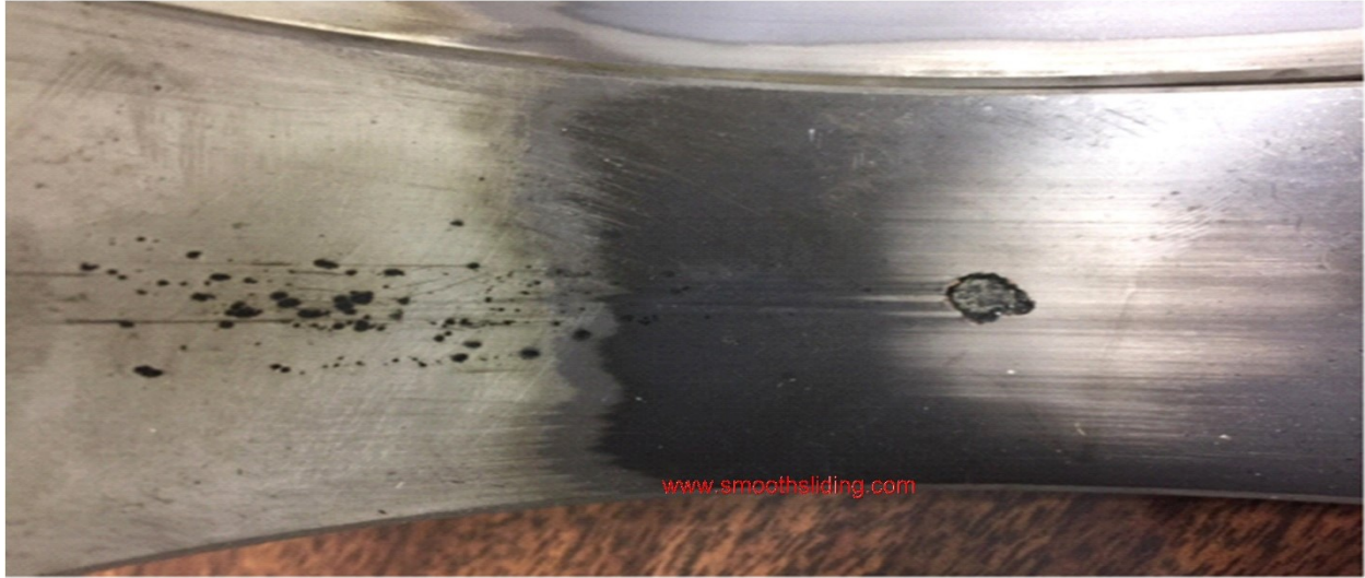
Fig.19 Corrosion of Lead in Heavy-Duty Engine Bearing
