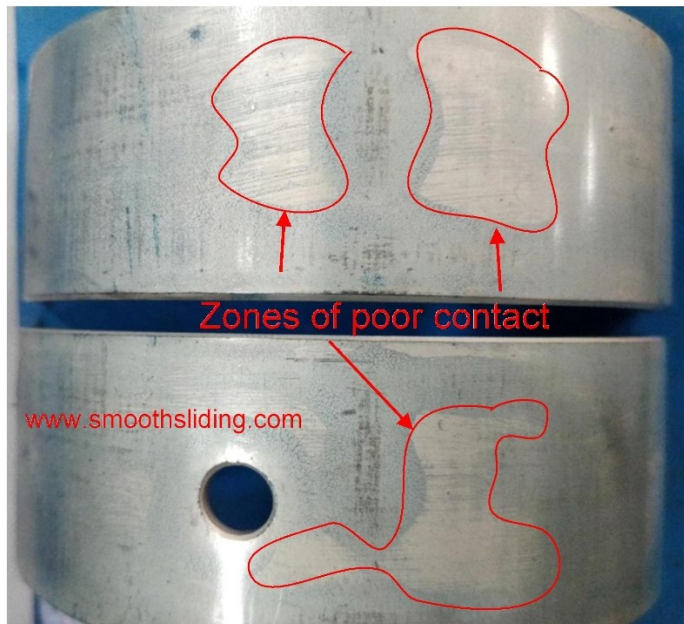
Fig.18 Poor Back Fitting of Heavy-Duty Rod Bearings
