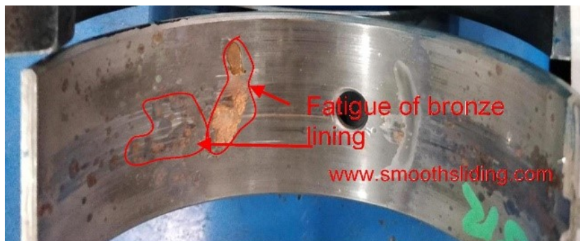
Fig.13 Fatigue of Bronze Lining of Heavy-Duty Rod Bearing
