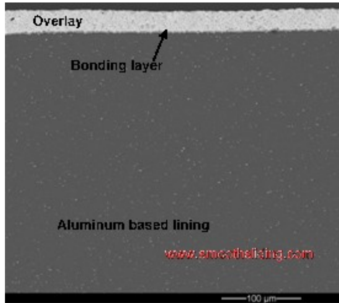
Fig.4 Structure of Trimetallic Heavy-Duty Engine Bearing with Aluminum Lining
