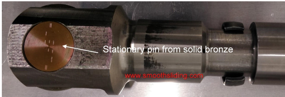
Fig.5 Valve Roller Lifter with Solid Bronze Pin
